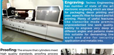
electronic engraving which are ideal for packaging, decor printing and uses sepecific filter for board and foil printing. Plenty of useful feactures like transcribe mode premits unprecedented line work quality. Ability to engrave very deep at different angles and patterns make this suitable for demanding line. this suitable for demanding line work and also for security application and metallic inks.
